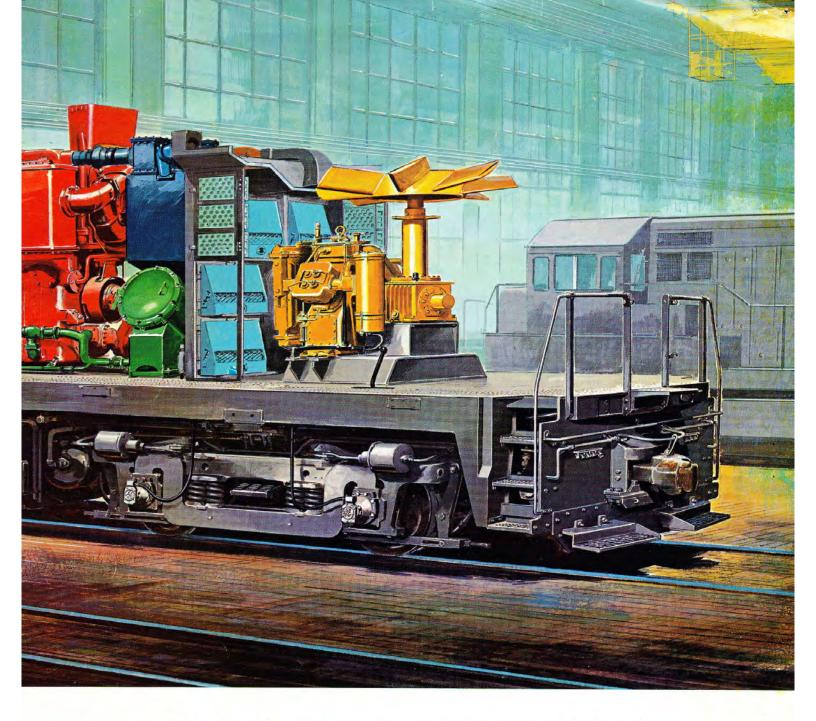
☐ The U33 with 3,300 horsepower gives railroads an opportunity to improve scheduled speeds or to increase hauled tonnage. Higher speeds over the grades are possible with full horsepower available over the locomotive speed range.
